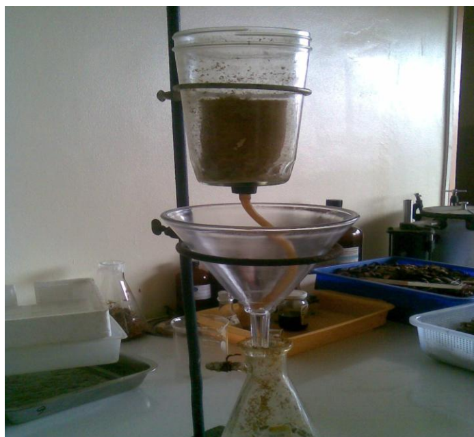
Figure 2 Maceration Set-up of Ground Acacia Bark
