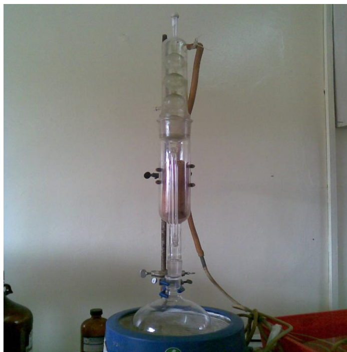
Figure 3 Extraction Using Soxhlet Apparatus
