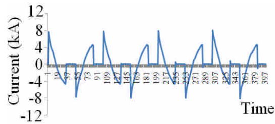
Figure 5. Current waveform from conditioning circuit.
