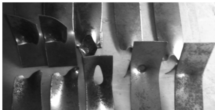
Figure 14(c). Tear from one side (PF) failures.
