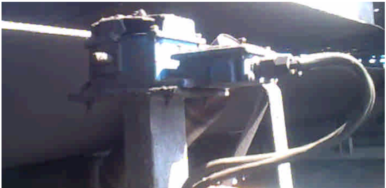
Fig.4. Image of Hydraulic control self-aligning-idler with displacement sensor
