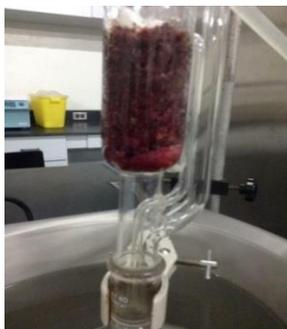
**Figure 2. Onion extraction using Soxhlet method**
