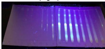
Figure 5. Chromatogram of fractions 2-35 under UV light
