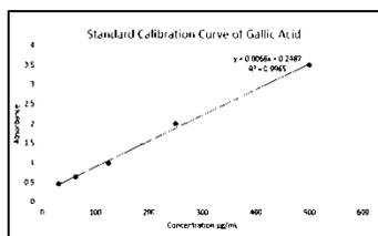
Figure 6. Standard Calibration Curve of Gallic Acid
