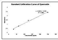
Figure 7. Standard Calibration Curve of Quercetin
