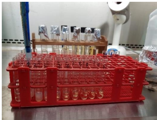
Figure 6. MIC determination through macrobroth dilution.
