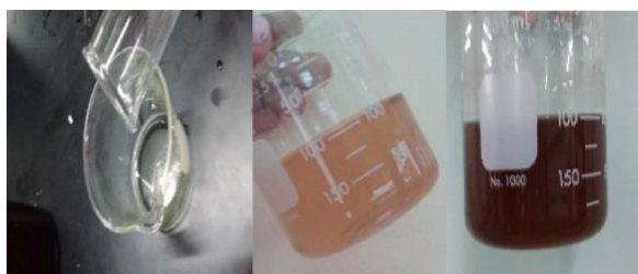
Figure 9. Color change in the synthesis of Ag NPs
