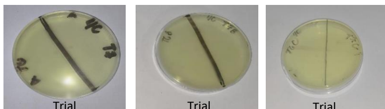
Figure 5. Bactericidal Concentration subculture on Mueller Hinton Agar showing no growth form the subcultured inoculum of Tube 6 and 7
